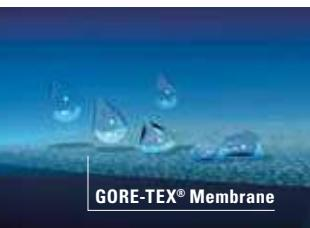
Durably waterproof and breathable GORE-TEX® shoes keep feet dry and provide optimized climate comfort. Core technology is the GORE-TEX® membrane whose microscopic pores are 20,000 times smaller than a drop of water, but 700 times larger than one vapour molecule. Water cannot penetrate while perspiration can easily escape.
